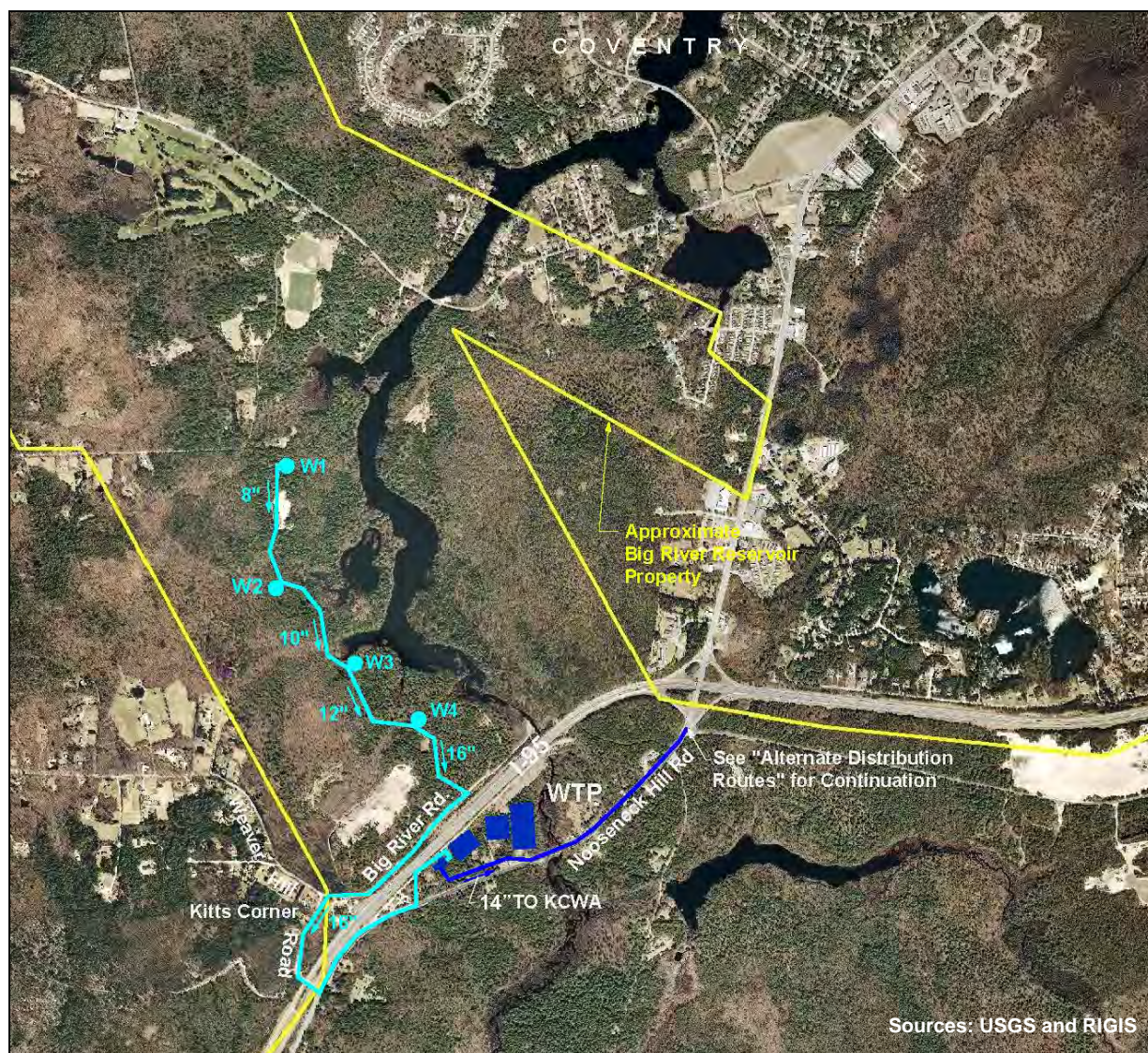
Figure 6: Conceptual Big River Water Treatment Plant and Well Development Scenario
